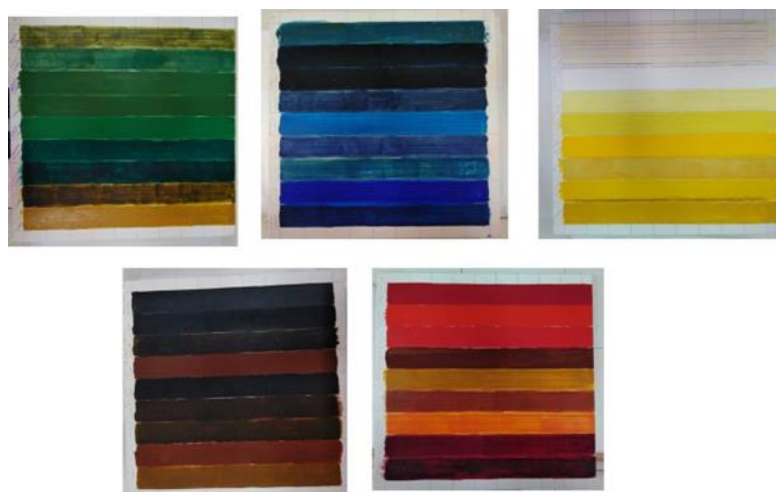
Figure S1. The 5 panels with single layer pigments on the preparation with: 1. green, 2. blue 3. white and yellow, 4. black and earthy and 5. red pigments are shown in order.
