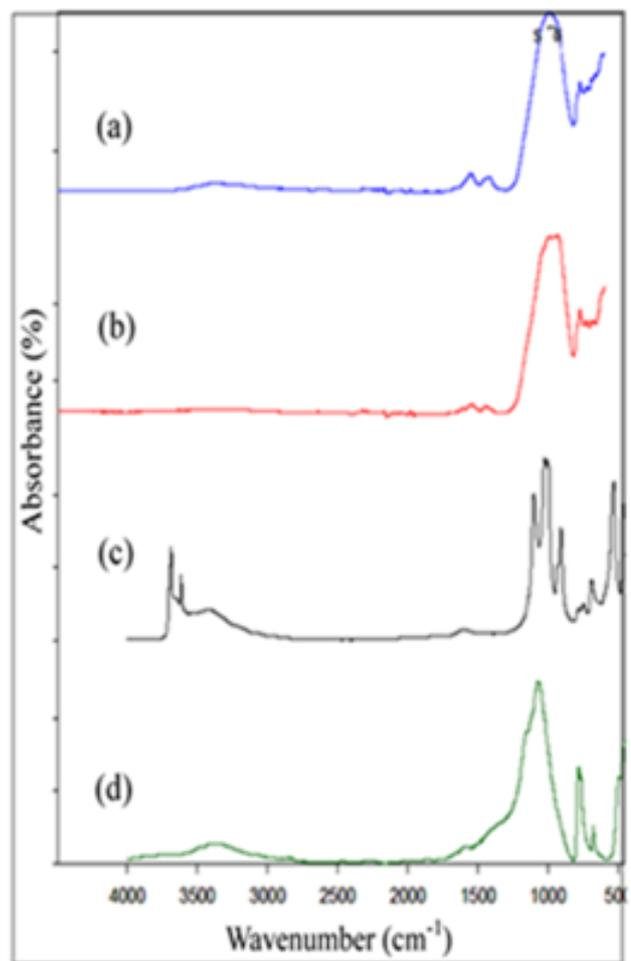
Figure 9. FTIR spectra of (a) the original slip (b) the silica reference sample (c) the original pottery (d) the kaolinite reference sample
