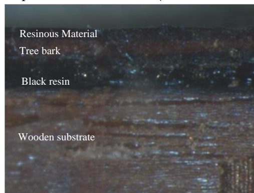
Figure 4. stratigraphic structure shows the sequence of the stick layers (Magnification 500x)
