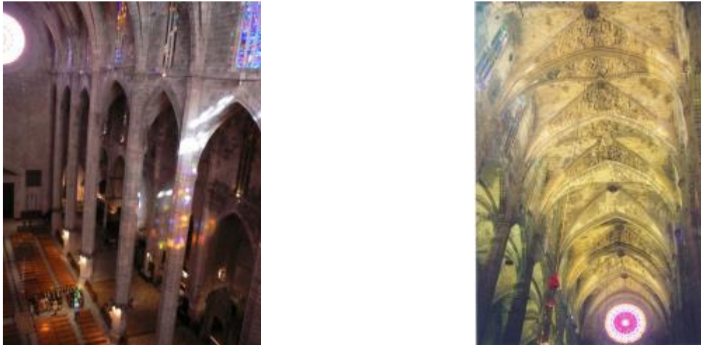
Figure 6. Internal views of Mallorca cathedral: looking at west façade and north nave, note the slenderness of columns and the upper and lower clerestories (left), and main nave vaults (right).
