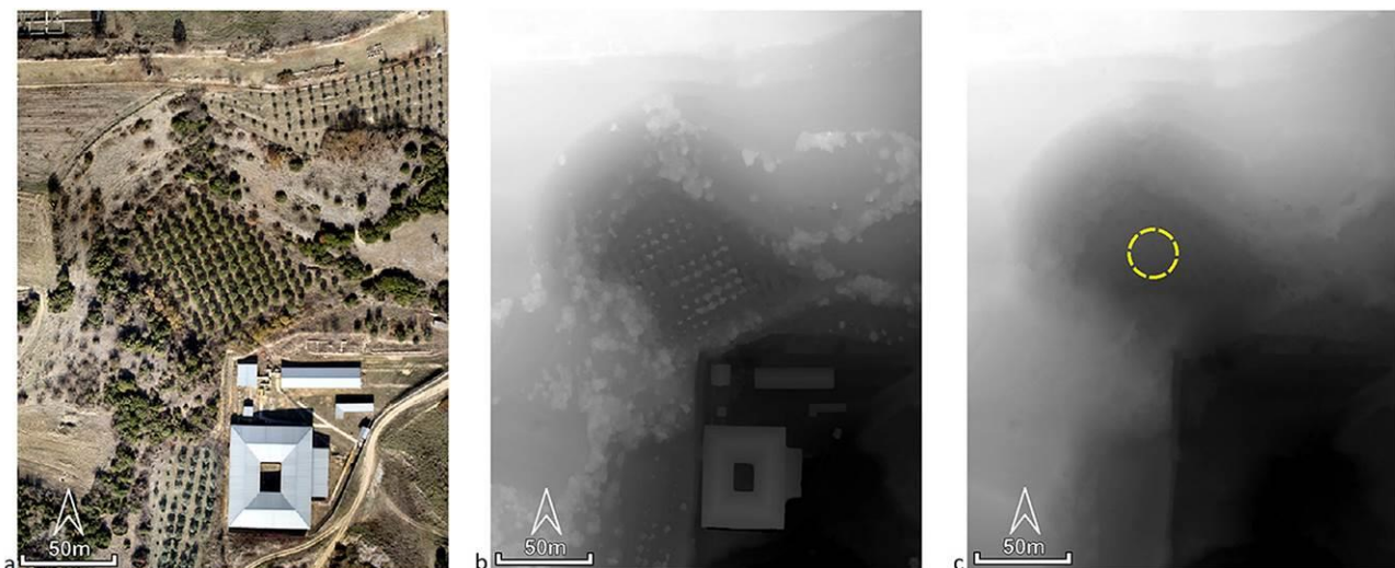
Figure 6. Products of the digital image processing of the Drone. a. Ortho image, b. Digital Surface Model (DSM), and c. Digital Terrain Model (DTM), with altitudes from 79.3m (black) to 123.5m (white), and the possible location (the research is in process) of the theatre's orchestra (yellow color). Spatial analysis of geospatial products of 3 cm (personal file).
