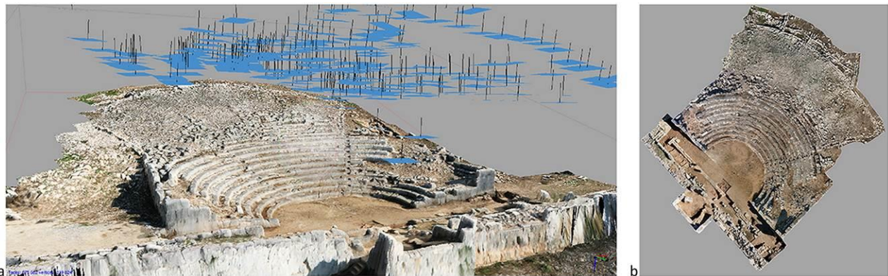
Figure 4. a. The 3D model of the ancient theatre of New Plevronas and the images' location (Agisoft PhotoScan®), b. ortho image (spatial resolution 1 cm) of New Pevronas (personal file).
