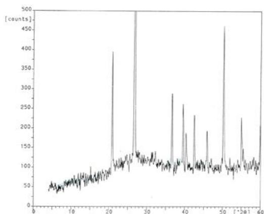
Figure 11. X-ray diffraction pattern of deteriorated red faience bead.
