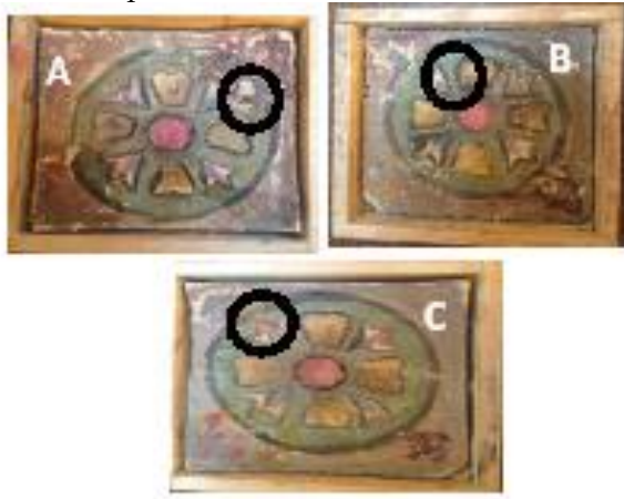
Figure 2 A, B and C, three models after cleaning with three kind of microemulsion filled in three kind of pulps.
