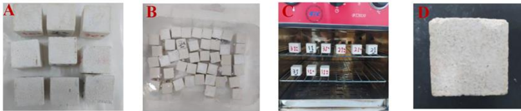
Figure 1. The experimental samples in industrial weathering cycles, where points (A) show the experimental samples before artificial aging, points (B-C) show the experimental samples during different industrial weathering cycles, and point (D) show the experimental samples after industrial Artificial aging.
