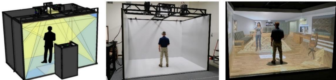
Figure 13: Specially designed multi-screen/projector VR example (CAVE -Automatic Virtual Environment- VR technology).
