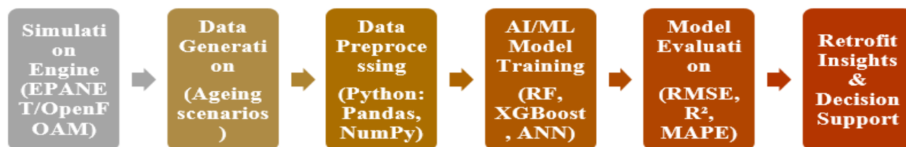
Figure 2: Analysis Flowchart (AI/ML-Integrated Predictive Modelling Framework).
