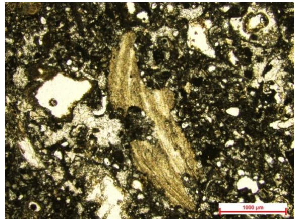
Figures 49. Photomicrograph of the studied limestone sample from Hussein Al-Refaie house
