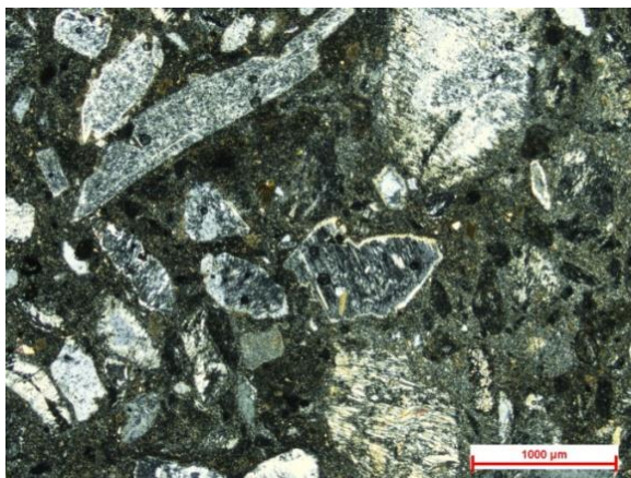
Figures 48. Photomicrograph of the studied mortar sample from Ahmed Al-Refaie house
