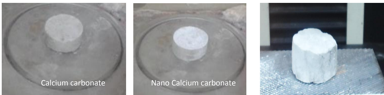
Figure 2. The samples of natural calcium carbonate, nano calcium carbonate and converted calcium hydroxide and the difference in color.
