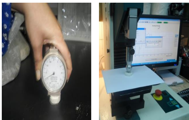
Figure 4. Testing samples for Hardness using Shore D and bursting strength test using Tinuis Olsen
