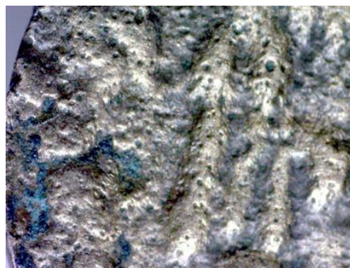
Figure 2. Magnified Image (x25) of Coin no. 2 , as an example of coins made by casting
