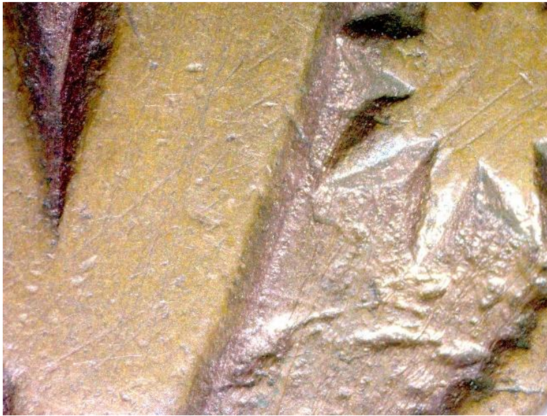
Figure 3: Magnified Image (x25) of Coin no. 6 As An Example of Coins Made by Striking
