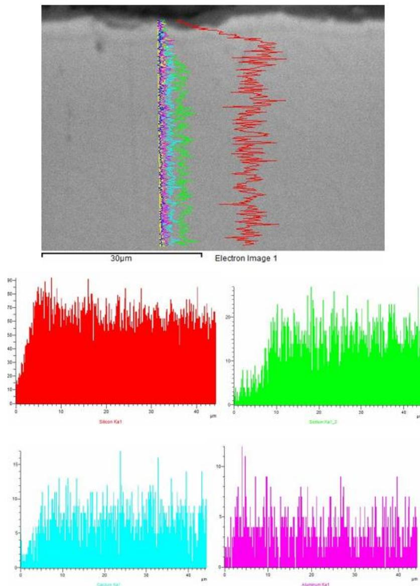
Figure 10. SEM-EDS Line Scanning Sample Man 7, core formed vessel, blue area. Graphs: red-silicon, green-sodium, aqua-calcium and violet-aluminum (0 µm: external surface)
