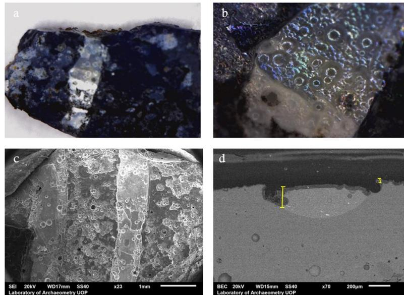
**Figure 9.** Sample Man 11: LED-OM Images *a* (up left) Iridescence (magnification  $\times 50$ ) and *b* (up left) iridescence and pitting (magnification  $\times 200$ ). SEM images *c* (down left) iridescence and pitting (magnification  $\times 23$ ) and *d* (down right) cross section of the sample. The lamination thickness appear to be 5-6 times thicker than at the blue body (magnification  $\times 70$ ).
