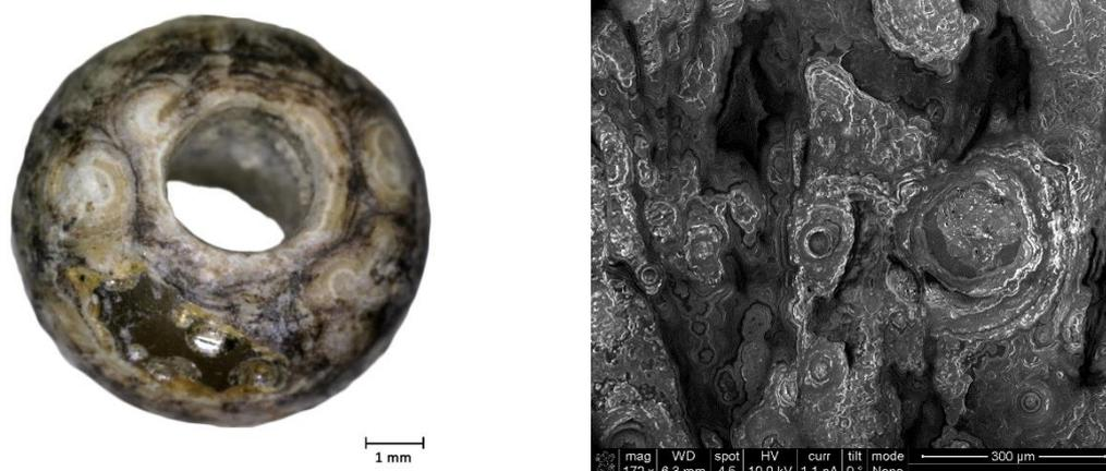
**Figure 7. Left: The surface of glass bead MEΘ 889-3 (Tomb 245/5) shows deterioration likely caused by microorganisms, in the form of groups of concentric circles and dark bands. Right: SEM images taken of the surface of bead MEΘ 884β shows evidence of deterioration due to microorganisms as both groups of concentric circles and circular holes.**
