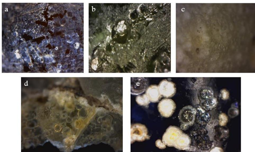
Figure 8. Identified corrosion patterns under LED-OM: a (up left) iridescence, b (up centre) pitting, c (up right) dark brown and black staining in white sample, d (down left) semi opaque milky like surface and e (down right) pitting with characteristic concentric layers forming local crust.
