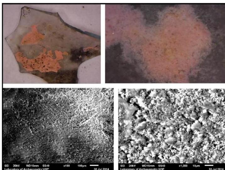
**Figure 3. LED microscope (Left: x10; Right: x50) and SEM images (Left: x100; Right: x1000) of the pink residue.**
