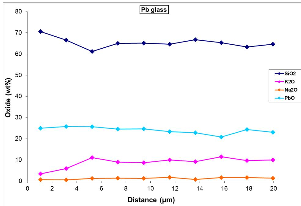
Figure 2. Representative concentration profiles of the main oxides, as determined by SEM/EDS, for K-rich glasses (up), Na-rich glass (middle) and high-lead glass (down) (0 μm: external surface).
