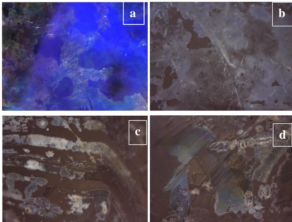
**Figure 1. Representative LED images (magnification x50) from surfaces showing iridescence (a), dulling (b), milky-like surface (c) and pitting (d)**
