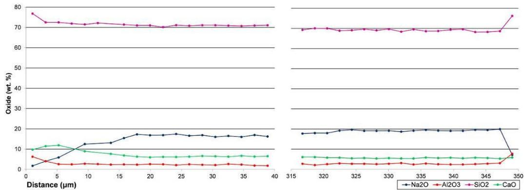
Figure 4. Concentration profile by SEM/EDS (0  $\mu\text{m}$ : Inner surface; 350  $\mu\text{m}$ : Outer surface).
