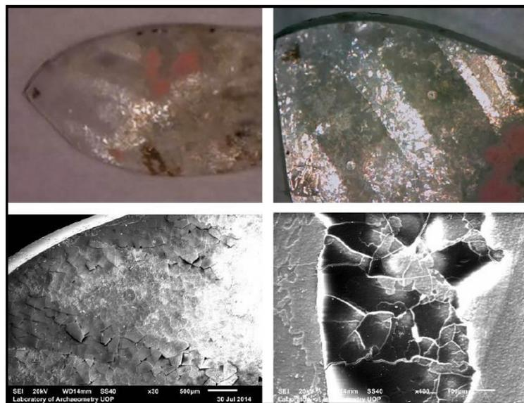
Figure 5. LED microscope (Left:  $\times 10$ ; Right:  $\times 50$ ) and SEM images (Left:  $\times 30$ ; Right:  $\times 100$ ) of iridescent layers on the inner surface of colourless fragments.
