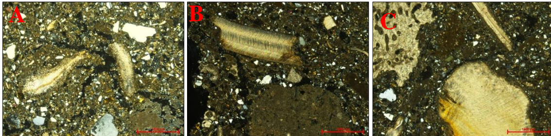
Figure 11. Examples of thin section photomicrograph of the structural mud-lime mortar samples taken from the outer layers and the inner filling layer of multiple-leaf masonry walls of the Al-Shafei mosque, (A and B) showing molluscan shell fragments with coarse quartz grains embedded in silty lime matrix, along with few fractures and voids, (C) showing coral skeletons, algal fragments and shell fragments and with few coarse quartz grains embedded in silty lime matrix.
