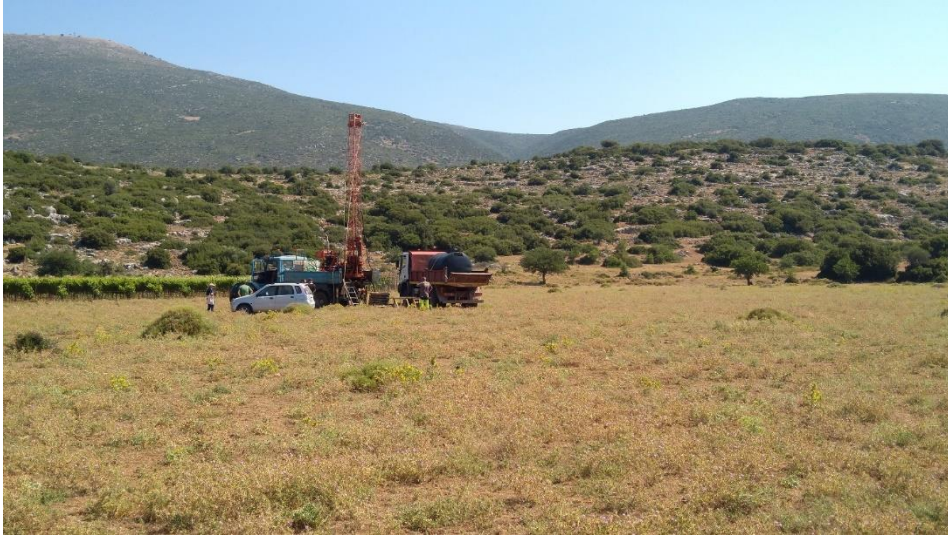
Figure 8. Boreholing for the investigation of the Meteles depression a and b) the boreholing trailer across kastrouli hill, c) extraction of cores, d) the cores (now properly stored in the premises of the University of Patras, attention of collaborators Prof. M.Geraga and Prof. G.Papatheodorou)
