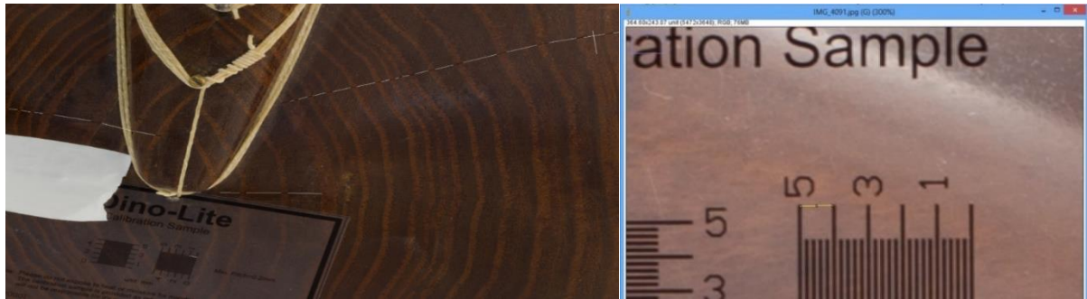
Figure 5. The process of taking photos, analyzing and measuring (using calibration sample)
