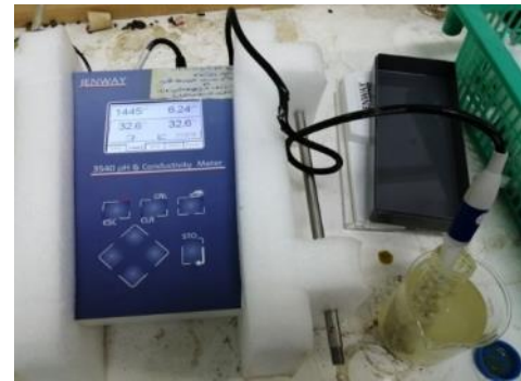
Figure 7. Measuring the PH Value by using Jenway Model 3540 pH/conductivity meter.
