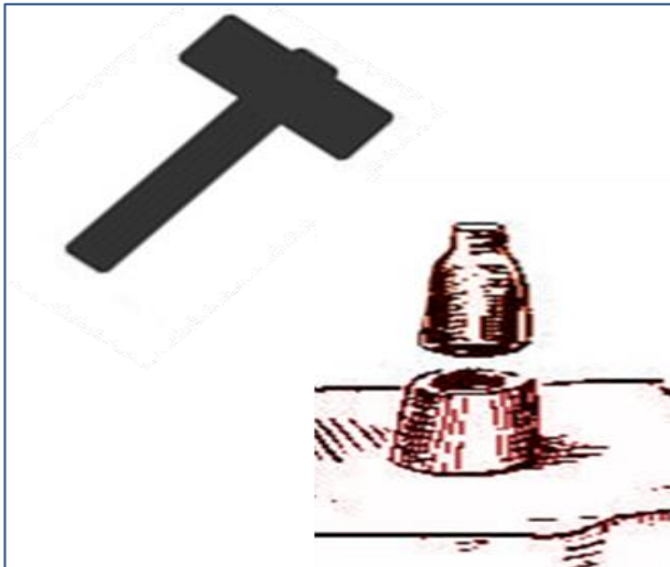
Figure 2 Schematic illustration of the process of striking or stamping flans
