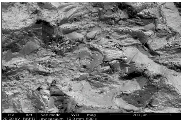
Figure 14. The SEM examination of the sample treated with Nano silica+ Wacker (OH 100) (500X).
