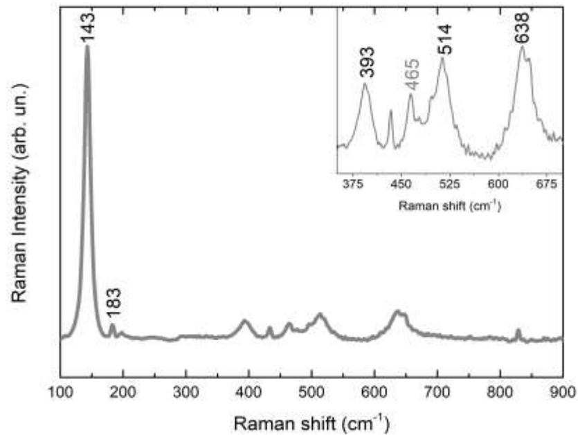
Figure 4: Raman spectrum (zoom inset) obtained for the white layer; typical Raman shift wavenumbers of anatase are highlighted in black numerals, while signals of quartz are evidenced in grey numerals.
