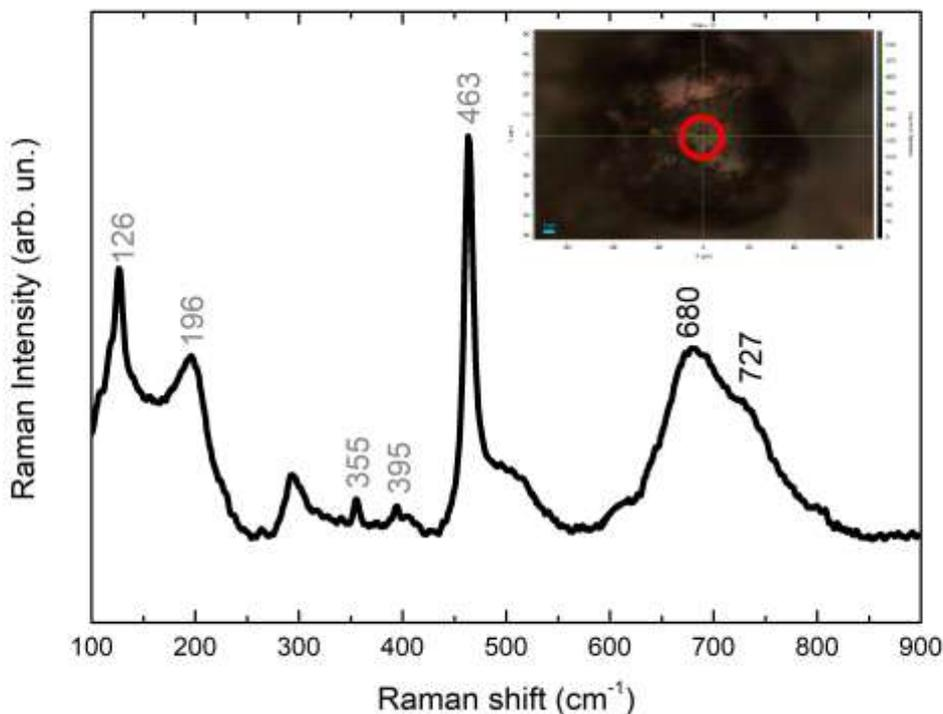
*Figure 3: Raman spectrum obtained for a brown-black particle (spectrum acquisition area evidenced by red circle in the inset); typical Raman shift wavenumbers of maghemite are highlighted in black numerals, while the quartz analogues are evidenced in grey numerals.*
