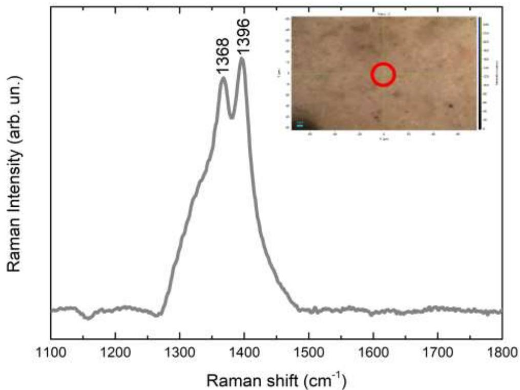
Figure 5: Raman spectrum obtained for the white layer (spectrum acquisition area evidenced by red circle in the inset); typical Raman shift wavenumbers of  $\alpha$ -alumina are highlighted in black numerals.
