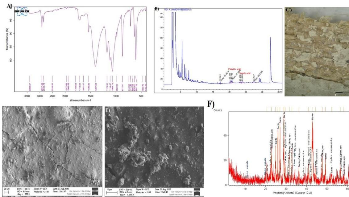
Figure 11. ATR- FTIR spectra of the powdered black paint A), GC-MS chromatogram of the binding medium B), C) stereomicroscope image mag x 3.2 of the ground layer on canvas support, D), E) secondary electron images of the ground layer, and F) XRD pattern of the ground layer.
