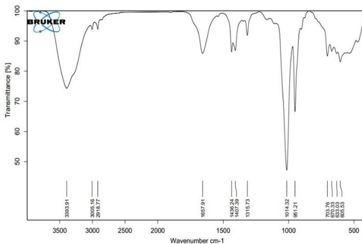
Figure 10. The peaks of ATR- FTIR spectrum of dammar varnish
