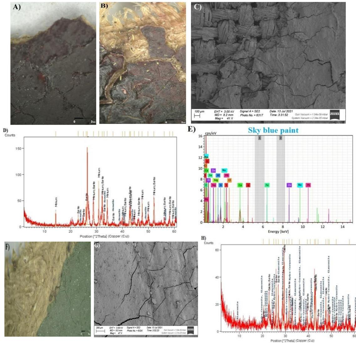
Figure 12. Microscopic examination of red paint A), B) stereomicroscope images mag x 3.2, C) Secondary electron image mag x 40, D) XRD pattern of red pigment, E) EDS analysis of sky blue paint, F) stereomicroscope image mag x3.2 of green and light green paint, G) Secondary electron image mag x 47 of green and light green paint & H) XRD pattern of light green pigment
