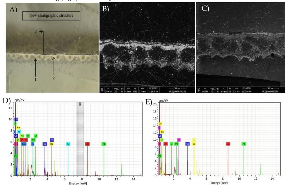
Figure 9. The new stratigraphic structure examinations a) stereomicroscope image mag x3, b) backscattering image mag x300, c) secondary electron image mag x 150, d) & e) EDS analyses of the olive green paint and ground layer respectively.
