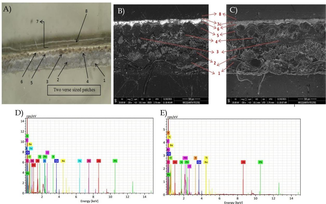
Figure 8. The original stratigraphic structure with the verse sized patches, A) stereomicroscope image mag x3.2, B), C) secondary electron and backscattering images mag x150, D) & E) EDS analyses of brown paint and ground layer respectively
