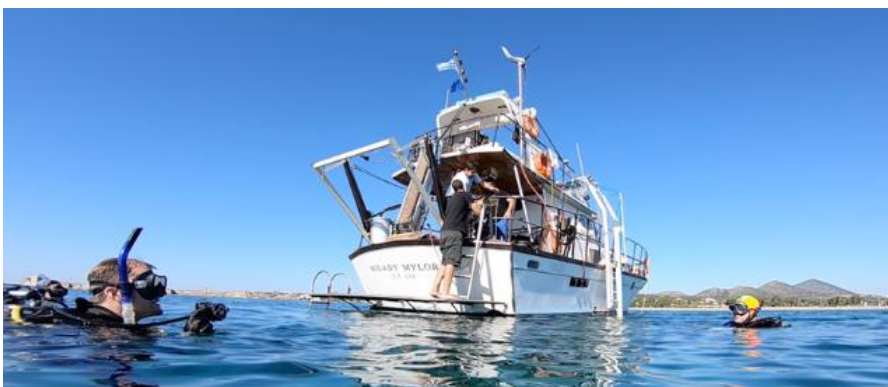
Figure 5. Research vessel, 'Mi-Lady My Lord' outfitted with sub-bottom profiler on right, multibeam, diving platform, and other instruments.
