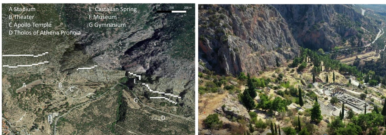
Figure 1. (left) Orthophoto of the archaeological site of Delphi. In this study, the rockfall reach probability is calculated for the locations marked with A-G (A: Stadium, B: Theatre, C: Apollo Temple, D: Tholos of Athena Pronoia, E: Castalian Spring, F: Museum, and G: Gymnasium). The white lines indicate the location of areas of potential rock detachment from the cliff (rockfall sources); (right) View of Phaedriades rocks and the sanctuary.
